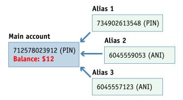
PortaBilling100 presents a new feature called "account aliases" where an alias serves as a link or pointer to the main account. When a customer uses an alias ID for authentication, PortaBilling retrieves information about the main account and uses its balance, product type and other parameters for all further operations.
