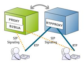
This allows to efficiently prioritize transmission of IP packets carrying the voice media and prevent any resource-intensive operations on the SIP side from affecting the voice quality.
