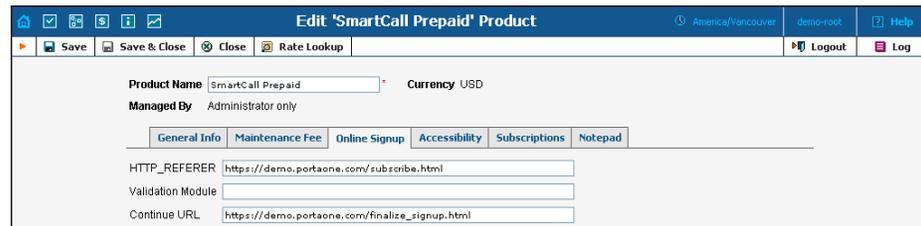
Numerous online signup frontends can be developed using a combination of the “HTTP\_REFERERER” and “Validation Module” fields.
