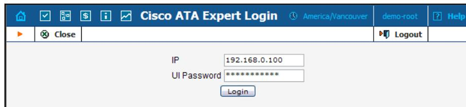
To edit configuration parameters, enter a UA IP address and password. The resulting screen will be similar to the UA Profile Management screen in the previous section.
